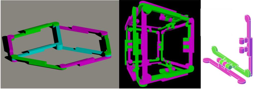
Fig. 5. On the left we introduce the mechanism that preserves the planarity and central symmetry of hexagonal faces. On the middle, we can see a CAD model of the cube ZSF. On the right three adjoining elements can be seen.
