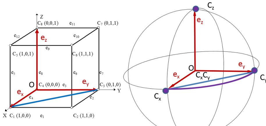
Fig. 4. On the left, a cubic mechanism can be seen that satisfies the planarity and central symmetry conditions having one diagonal brace on the base face. On the right, we can see the corresponding auxiliary framework. The end of base unit vectors and the arc form the rigidity graph  $G_{ZSF}$ .
