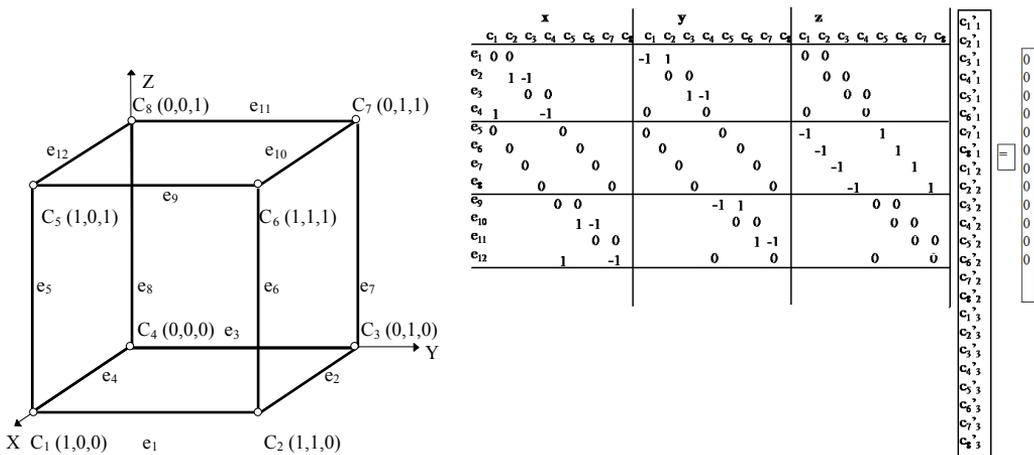
Fig.2. On the left we can see a cubic bar-and-joint framework, which is not a special one, generally the four of the joints of a square faces can move to a skew rhomb. The solution of the system of equation- on the right determines the possible infinitesimal motions.
